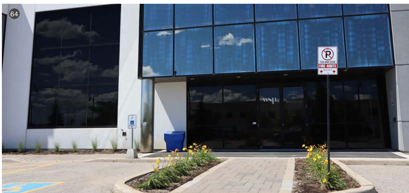
Site design should facilitate comfortable pedestrian access and circulation between sidewalks, parking areas and building entrances
